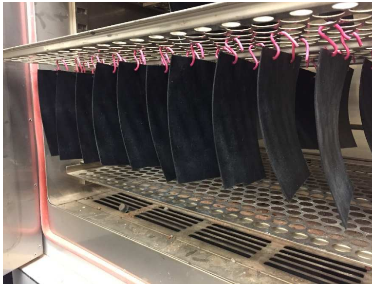
Figure 6.4 A view of the HDPE GMB sheets inside the air forced oven
