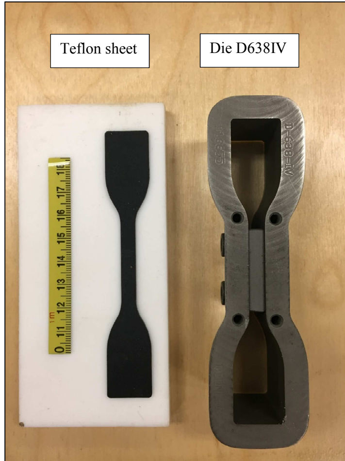
Figure 3.1 Teflon sheet and Pioneer die mold that used to cut dogbone geomembrane specimen
