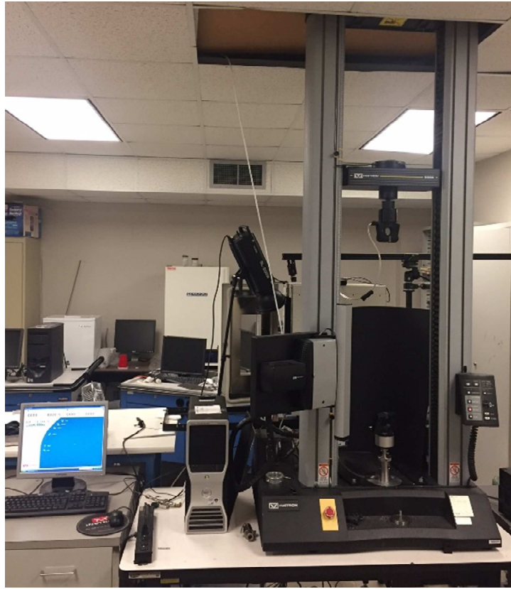
Figure 3.5 Experimental setup using an Instron 5566 and an Instron AVE video extensometer
