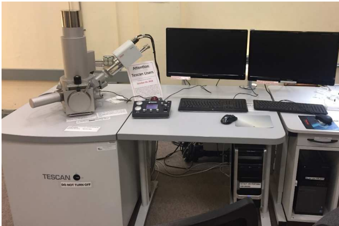
Figure 4.6 Tescan Vega-3 scan electron microscopy for imaging break surface of specimens
