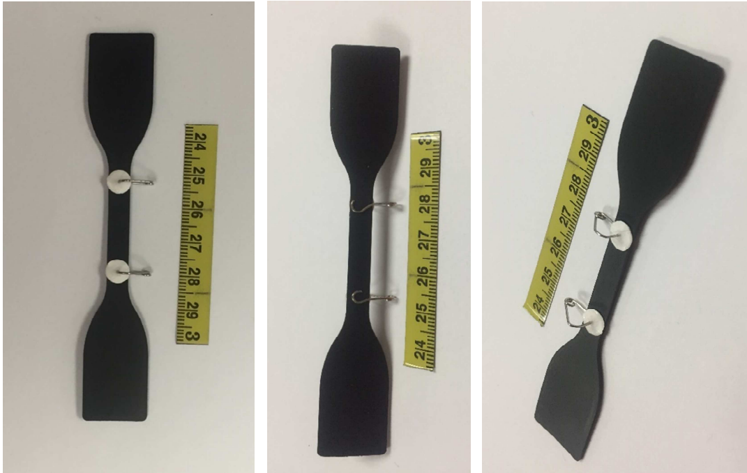
Figure 5.5 Center dot attached to a geomembrane specimen
