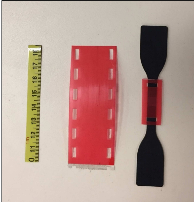
Figure 3.3 Preparing stick tape with a rectangular punched hole to locate gage marks
